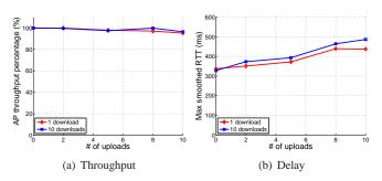
Fig. 5. Performance of the eBDP algorithm as the number of upload flows is varied. Data is shown for 1, 10 download flows and 0, 2, 5, 10 uploads. Wired RTT 200ms. Here the AP throughput percentage is the ratio between the throughput achieved using the eBDP algorithm and that by a fixed buffer size of 400 packets (i.e. the maximum achievable throughput in this case).
